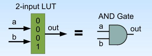
\* 3000 transistors per LUT (incl. routing config bits); LUT == 5 gates
