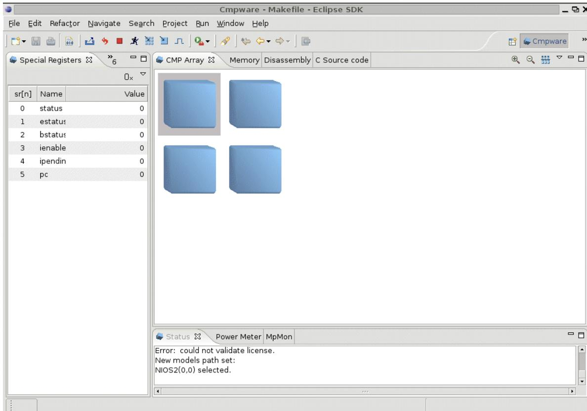
**Figure1:** The *Cmpware CMP-DK* default screen.
